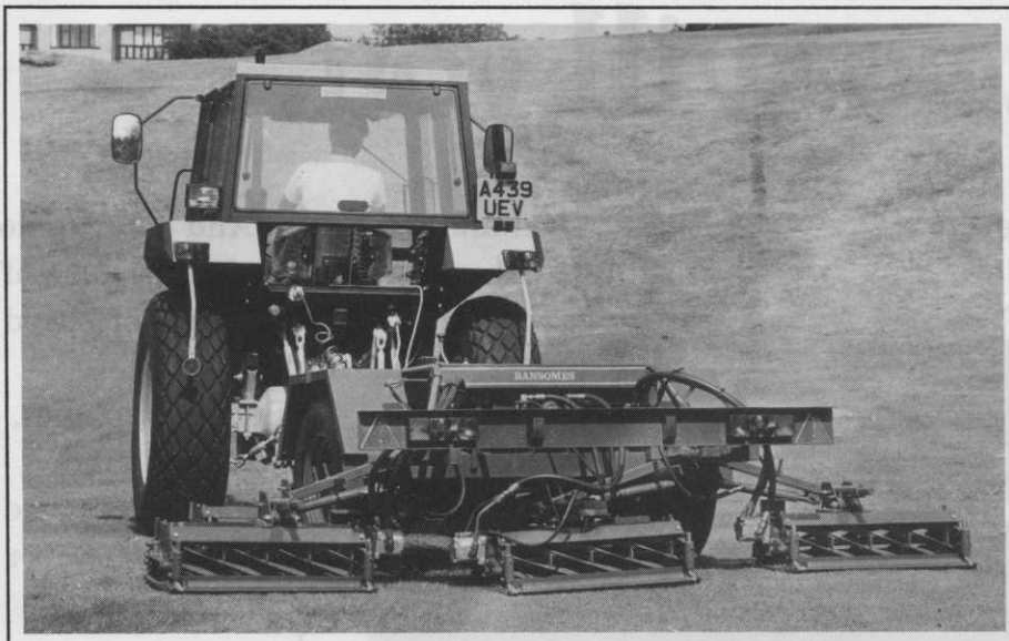
Pictured cutting a fairway is a Ransomes Hydraulic 340TG trailed gang mower with 8-knife floating head cutting units
