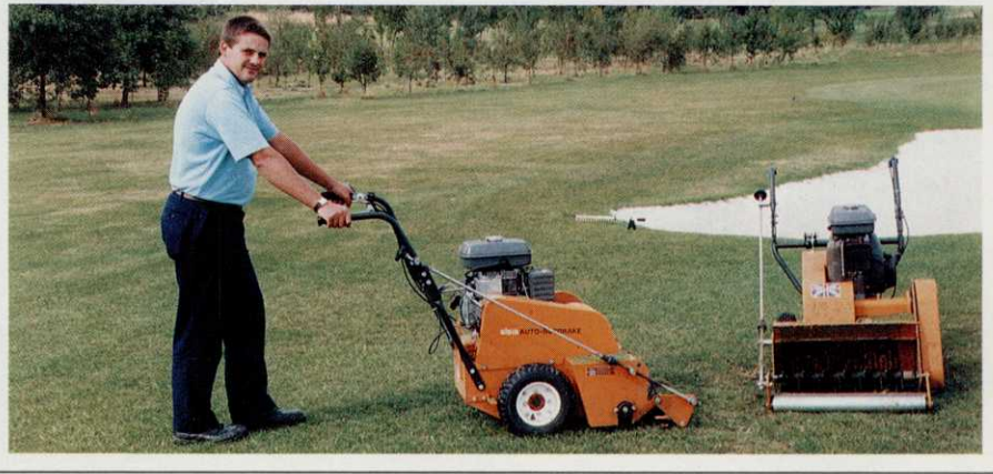
Head Greenkeeper Sam Hagan with the two Sisis Autorakes used to scarify the greens
