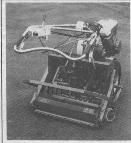
**S**ISIS introduced two new seeders, the first called the Contra-Seeder is pto driven and combines the SISIS principle of contra-rotating knives with the Auto-Seeder principle of accurate placement. Final testing of the Contra-Seeder was carried out at leading Manchester soccer grounds with the complete end-of-season re-seeding of their pitches. The operating width is 50ins. and the
