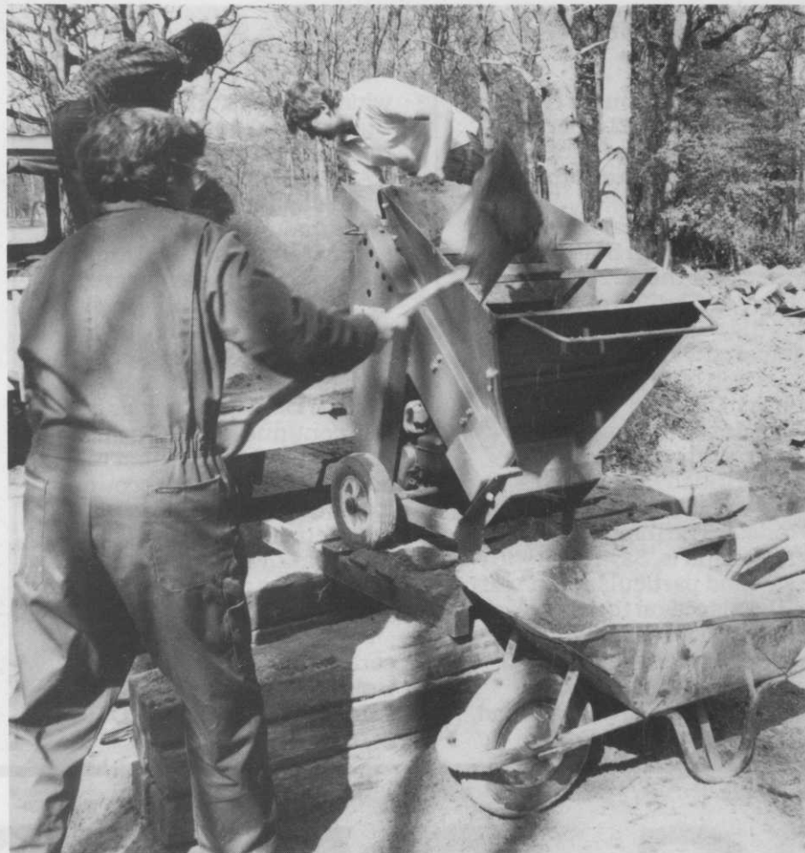
Bulk mixed soil and sand is loaded into the Royer 112. The shredder mixes, cleans and aerates the material before 'firing' it into a trailer ready for spreading. The club also uses a Royer Model 30 Powerscreen when grading or pre-cleaning is required.
