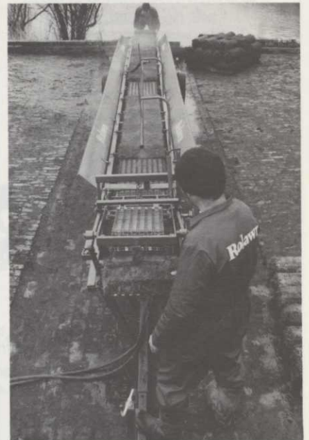
Britain's first automatic turf washer uses water from the river to direct high pressure, high volume jets to remove soil from beneath the Rolawn turves.
