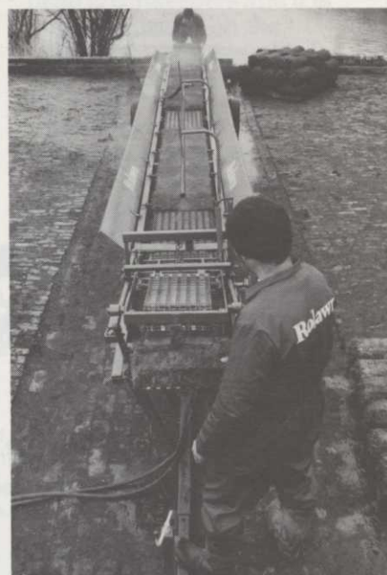
Britain's first automatic turf washer uses water from the river to direct high pressure, high volume jets to remove soil from beneath the Rolawn turves.
