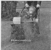
The build-up of a fibrous growth of dead material, known to the professional as "thatch", at the base of fine grasses, leads to a poor playing surface. Using any of the SISIS Rotorakes, thatch can be removed and a thatchfree playing surface maintained thereafter. Three reels are available to provide year round use of the machines - thatch removal reel, for cutting out accumulations of thatch; thatch control reel, for severing horizontally
