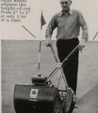
Dual control. Separate landroll and reel clutches enable easy control of the mower at all times.
