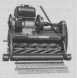
Brush and Comb Set. A nylon brush and steel comb are optional extras, for controlled turf grooming.
