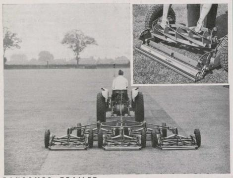
RANSOMES TRAILED GANG MOWERS. From single-unit (30 in.) to nine-unit (20 ft. 6 in.) cutting widths. Choice of "Sportcutter" units for close cutting, or "Magna" units for rougher work. Cutting cylinders can be removed without dismantling unit.
