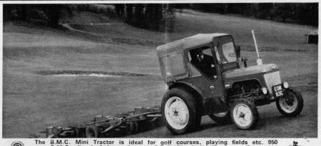
The B.M.C. Mini Tractor is ideal for golf courses, playing fields etc. 950 c.c. B.M.C. diesel, 9 forward gears P.T.O. live hydraulics etc. Get on to Gibbs for demonstration.
