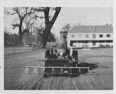
P.J.M. Sprayers have introduced a new model, GPS 60, easily adaptable for spraying Chlordane as well as selective weedkillers. The towed sprayer provides high or low volume at a constant rate of delivery between 3 and 10 m.p.h. Tank capacity is 60 gallons and the new double-barrelled 9 ft. boom will spray 45, 50 or 60 gallons per acre with alternative jets.
