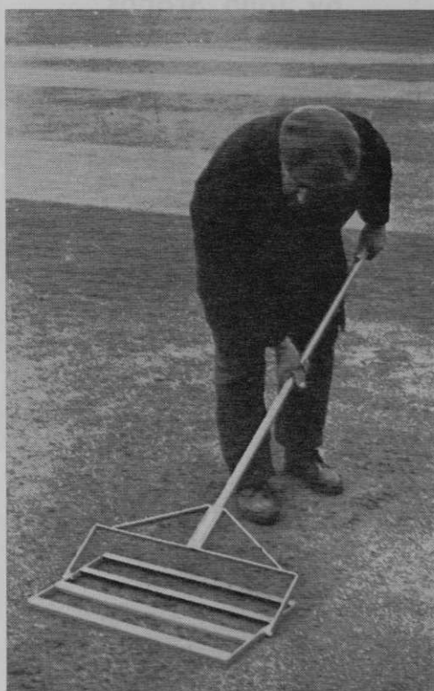
The new Sisis "TRULUTE" rubbing in top-dressing on a cricket wicket. The cutting edge is in action.
