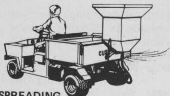
SPREADING Spreads 40' wide
