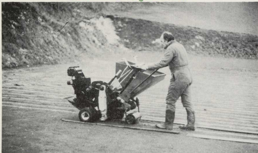
Single Blade Sand Injector operating on a Golf Green
