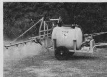
This 44 gallon trailer sprayer unit with its 18ft spray boom is perfect for the large park or golf course. Many useful accessories are available including a trolley sprayboom for working on fine turf up to 120ft away from the tractor.
