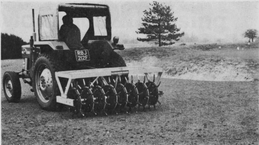
The Ransomes Hahn TM 80 Aerifier in action
