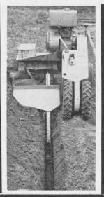
electric, telephone, and signal cables, water, gas, and oil pipes, sportsfield, and parks drainage
