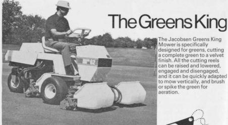
The Jacobsen Greens King Mower is specifically designed for greens, cutting a complete green to a velvet finish. All the cutting reels can be raised and lowered, engaged and disengaged, and it can be quickly adapted to mow vertically, and brush or spike the green for aeration.
