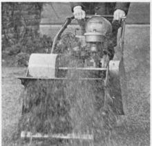
The build-up of a fibrous growth of dead material, known to the professional as "thatch", at the base of fine grasses, leads to a poor playing surface. Using any of the SISIS Rotorakes, thatch can be removed and a thatch-free playing surface maintained thereafter. Three reels are available to provide year round use of the machines—thatch removal reel, for cutting out accumulations of thatch; thatch control reel, for severing horizontally growing grasses, preventing the build-up of thatch; wire
