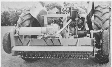
Two Vertirake Models for thatch removal on fine turf and out fields
