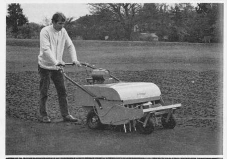
The new SISIS Autocrat is the ideal aerator for all fine turf areas — golf greens, bowling green, etc. The Autocrat gives fast coverage because of its great manoeuvrability (turns in its own length) its 3 ft. width and its speed of operation. A 600 sq. yd. golf green can be tined in 30 minutes and an average bowling green in  $1\frac{1}{2}$  hours.
