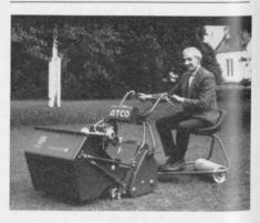
Atcokick start version of the 28 in. Groundsman. It is powered by a 256 cc 4-stroke engine with fan cowl cooling and fitted with a centrally positioned kick start lever and open handles to permit easy access to the starter in pedestrian use. The six heavy duty blades give 81 cuts per yard.
