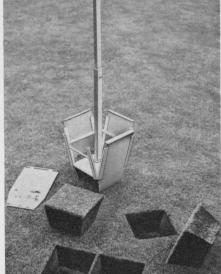
Square shape means unlimited adjacent cuts for any size of patch. No 'in-between' spaces as with round cutter.
