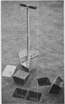
Square shape means unlimited adjacent cuts for any size of patch. No 'in-between' spaces as with round cutter.
