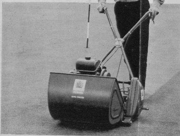
**Dual control.** Separate landroll and reel clutches enable easy control of the mower at all times.
