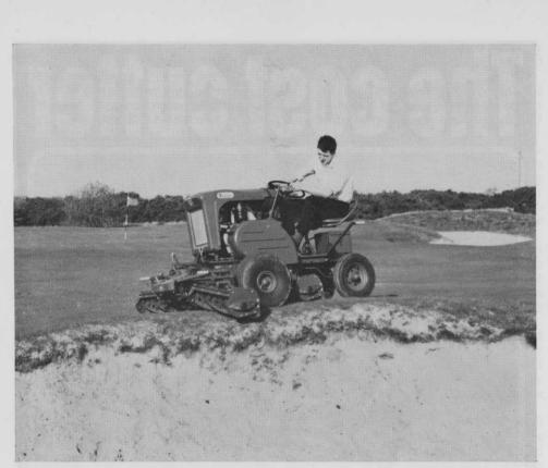
RANSOMES The Motor Triple Mower trimming the back of a golf course bunker.
