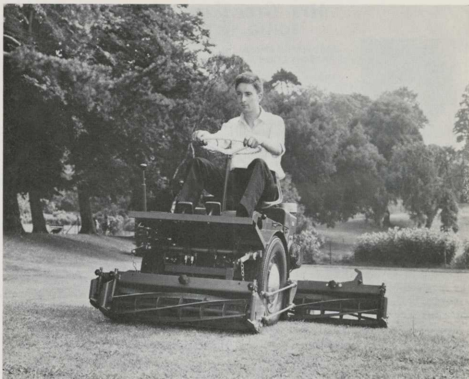
The new JUNIOR MOTOR TRIPLE from Ransomes with three power driven units cutting 73" wide and up to 1¼ acres an hour.
