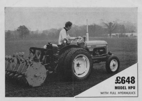
Nuffield 4/25 Tractor with "Sisis" 6ft. heavy duty aerator ref. H.A.6. The Wettest conditions can be overcome by fitting twin rear wheels as shown (rarely necessary).
