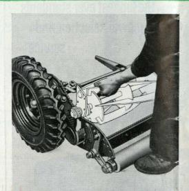
Easily removable cutting cylinders on Ransomes Gang Mowers save service time—add cutting time
