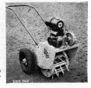
**PENETRATION** Will give up to 4" consistent depth of vertical clean hole at 4" Pitch.
