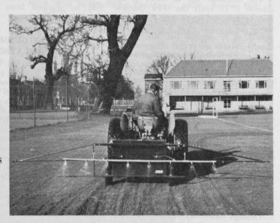
P.J.M. Sprayers have introduced a new model, GPS 60, easily adaptable for spraying Chlordane as well as selective weedkillers. The towed sprayer provides high or low volume at a constant rate of delivery between 3 and 10 m.p.h. Tank capacity is 60 gallons and the new double-barrelled 9 ft. boom will spray 45, 50 or 60 gallons per acre with alternative jets.
