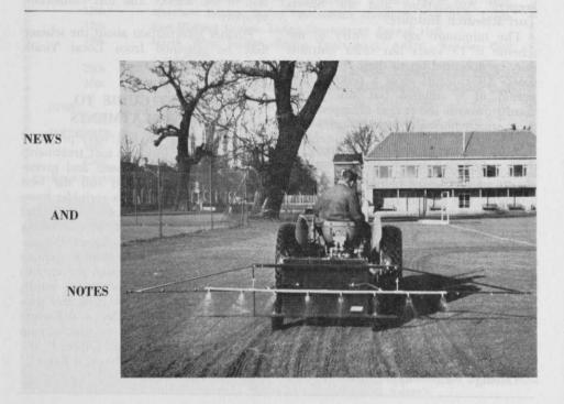
P.J.M. Sprayers have introduced a new model, GPS 60, easily adaptable for spraying Chlordane as well as selective weedkillers. The towed sprayer provides high or low volume at a constant rate of delivery between 3 and 10 m.p.h. Tank capacity is 60 gallons and the new double-barrelled 9 ft. boom will spray 45, 50 or 60 gallons per acre with alternative jets.
