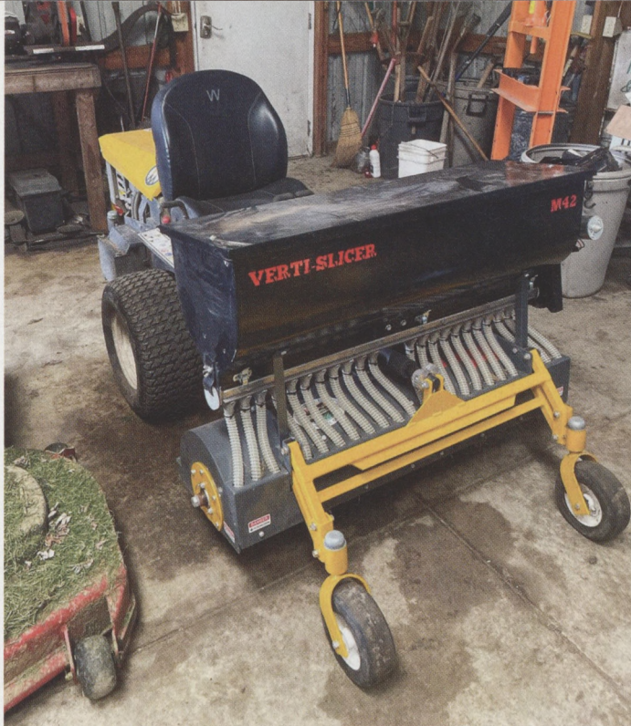
Fran Meister attaches a 42-inch slicer seeder to his zero-turn mower to create a fall overseeding workhorse.
