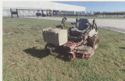
Scott Hord attaches spray tanks to some of his zero-turn mowers so operators can spot spray as they mow.
