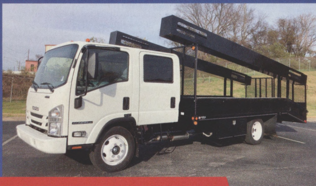
19' Irrigation w/Pipe & Fitting Boxes
