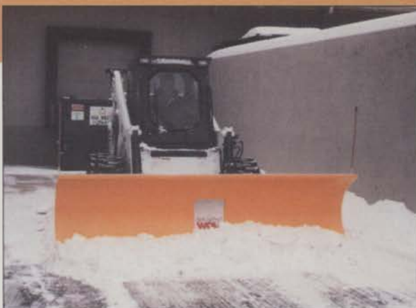
Plowing with a skid-steer loader allows contractors improved maneuverability, access to cramped areas and sturdy clearing power.
