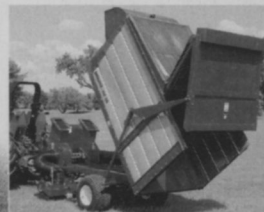
Model BV138 features hydraulic lift unloading
