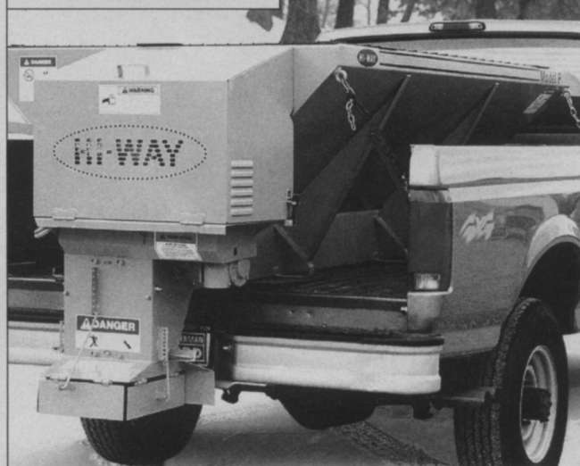
Model P Deicing Spreader for winter salt and sand application
