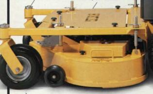
18"x 8.00" turf-tread drive tires, the largest on any walk-behind anywhere, for a smoother ride, better flotation, and reduced psi
