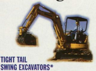
Horsepower: 18.7 HP@2600 rpm - 37.8 HP@2500 rpm Digging Depth: 7'9" - 11'2" Operating Weight: 5050 lbs. - 9880 lbs.
