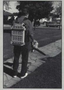
Equipped with a nickel metal hydride battery, Echo's new alternative energy power blower provides consistent power for about 40 minutes. Photo: Echo
