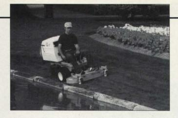
In addition to the maneuverability benefits of some riding mowers, contractors have shown an appreciation for visibility mid-mount mowers afford the operator for trimming purposes or mowing along edges. Photo: Walker Mfg.
