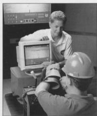
Operators can simulate the use of a directional boring machine on this system.
