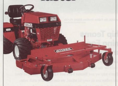
The new Steiner MX460 Mulching Deck does much more than the average mower. Six blades cut grass so finely, it decomposes quickly to nourish your turf. Smooth-rolling front caster wheels and a full-length rear roller precisely follow the lay of
