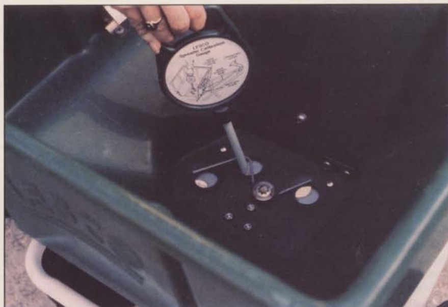
Figure 1. Calibration of a professional rotary spreader using a calibrating pin provided by the manufacturer.
