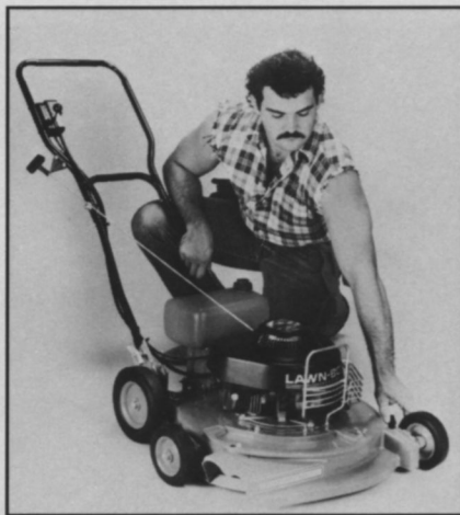
The remote pull-cord positioning is one safety feature incorporated in many commercial mowers.
