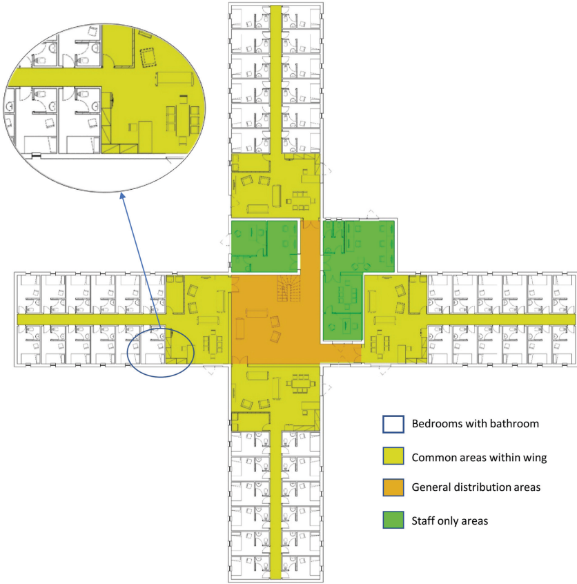
Figure 4.1 Typical blueprint of the Norwegian model 2015 for prison design. Outlining made by the Chilean architect Andrés Rodríguez-Ravanel, with guidance from the author based on the information collected in interviews and prison visits during the fieldwork
