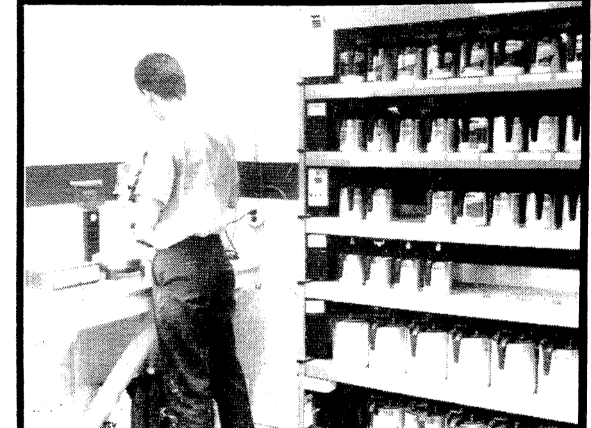
Bringing technology to the Collision business: Bill checks the paint formula on microfiche, weighs it (to .1 gram) and uses the 8-10 toners required to make just the right color for your vehicle.
