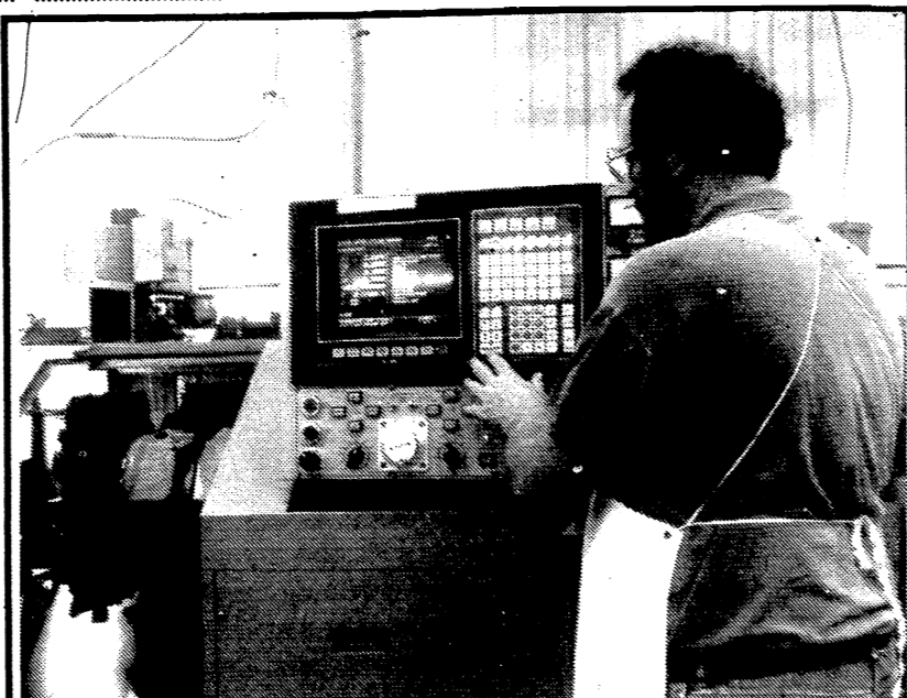
Pictured above, a computer programmer setting up and checking the program in anticipation of running a new job on a CNC milling machine.
