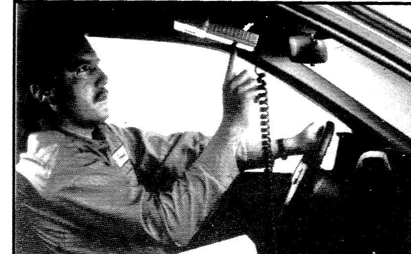
The Portable Vehicle Analyzer allows the dealer technician to electronically record engine data during a test-drive to identify hard-to-find problems.
