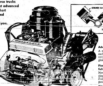
ldvanced aircraft-type valves new valve train design permits each valve to function independently-as in modern aircraft en-
