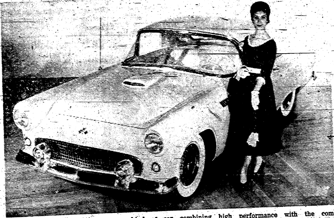
THE THUNDERBIRD, a new kind of car combining high performance with the comfort, convenience and safety of a conventional model, has been added to the Ford line. The Thunderbird has a powerful 160 h.p. Y-block V-8 engine and its low, graceful body is of all-steel construction. Equipped with a convertible cloth top which folds completely out of sight behind the rear seat, the Thunderbird can be purchased with a special composition hardtop, making it a complete all-weather car. Its overall height is 51.5 inches—nearly a foot lower than the 1954 Ford sedan—yet it has only slightly less road clearance. Most of its major parts are interchangeable with Ford's regular line of cars. The Thunderbird is scheduled for production by Ford Division next fall.
