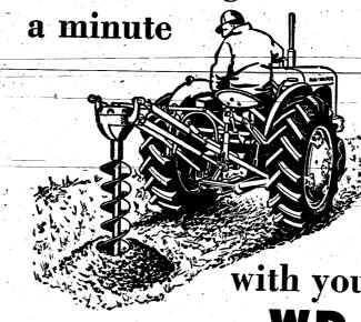
This combination of WD power and the Danuser Digger takes the work out of hole digging — whether for fence posts, poles, seedlings or construction work. This well-proved digger now mounts directly on the WD Tractor ... is driven through the power takeoff, and controlled by the tractor's hydraulic system It's a one-man, easy-to-operate tool, adapted especially for use with the WD Tractor. Ball-joint mountings prevent damage when passing
