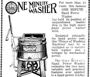
used exclusively in this The secret of the easy running of the Minute Washer is the high speed fly wheel. This fly wheel is mounted on a ball bearing and a very heavy standard close up under the bottom of the tub out of the way and is the source of the great pulling power that so wonderfully assists the user in operating the machine. By leans of the compound lever, the power is trebled, an
