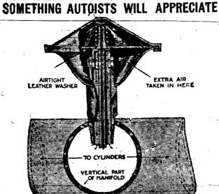
A COMPENSATING VAPOR PLUG WHICH AUTOMATICALLY ADMITS
