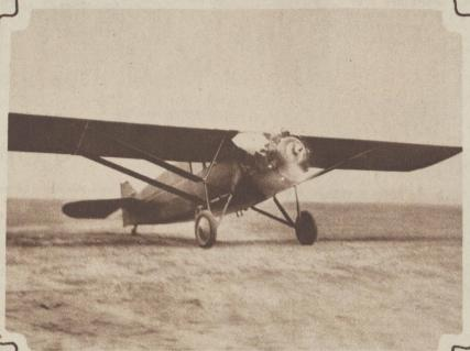
OIL BURNING AIRPLANE MOTOR-The new Packard Diesel motor, which burns the common variety of fuel oil, is foremost among the developments in airplane motors during the last year. Recent test flights show that it gives a greater cruising radius and consumes less fuel.
