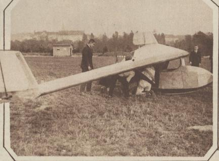
TAILLESS PLANE-This plane and another of the same type were flown successfully at Dessau, Germany, by Pilots Espenlaub and Groenhoff. The plane weighs 480 pounds and attains a speed of seventy-five miles an hour. It is propelled by a ten horsepower motor.
