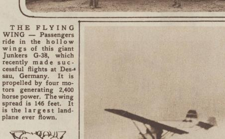
recently made successful flights at Dessau, Germany. It is propelled by four motors generating 2,400 horse power. The wing spread is 146 feet. It is the largest landplane ever flown.
