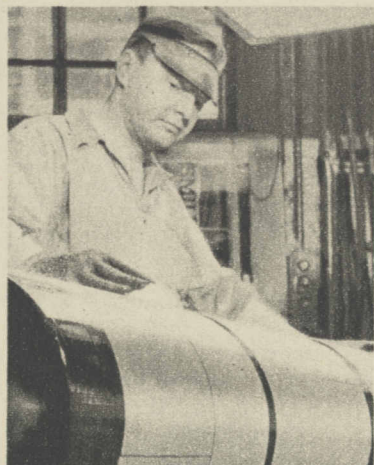
Etching a copper cylinder in the roto plant for use in printing the Picture and Graphic Sections.
