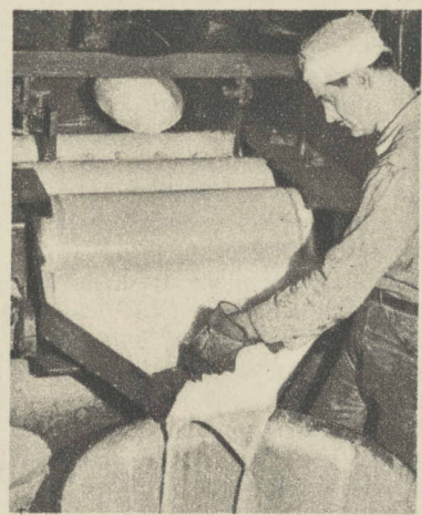
Blending colors to make the high-grade ink used in printing Tribune color pages. (Tribune photos.)
