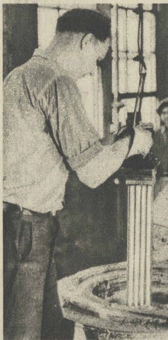
4 At the same time molds are made by dipping steel shaped to the desired form into molten lead, which "freezes" and is peeled off.
