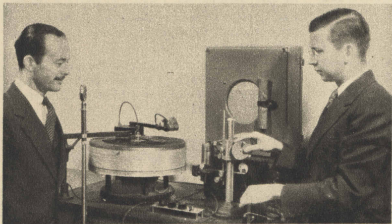
Professor Tiffin, right, photographs voice of Professor Steer, using the vibrograph which produced oscillogram pictured on this page.
