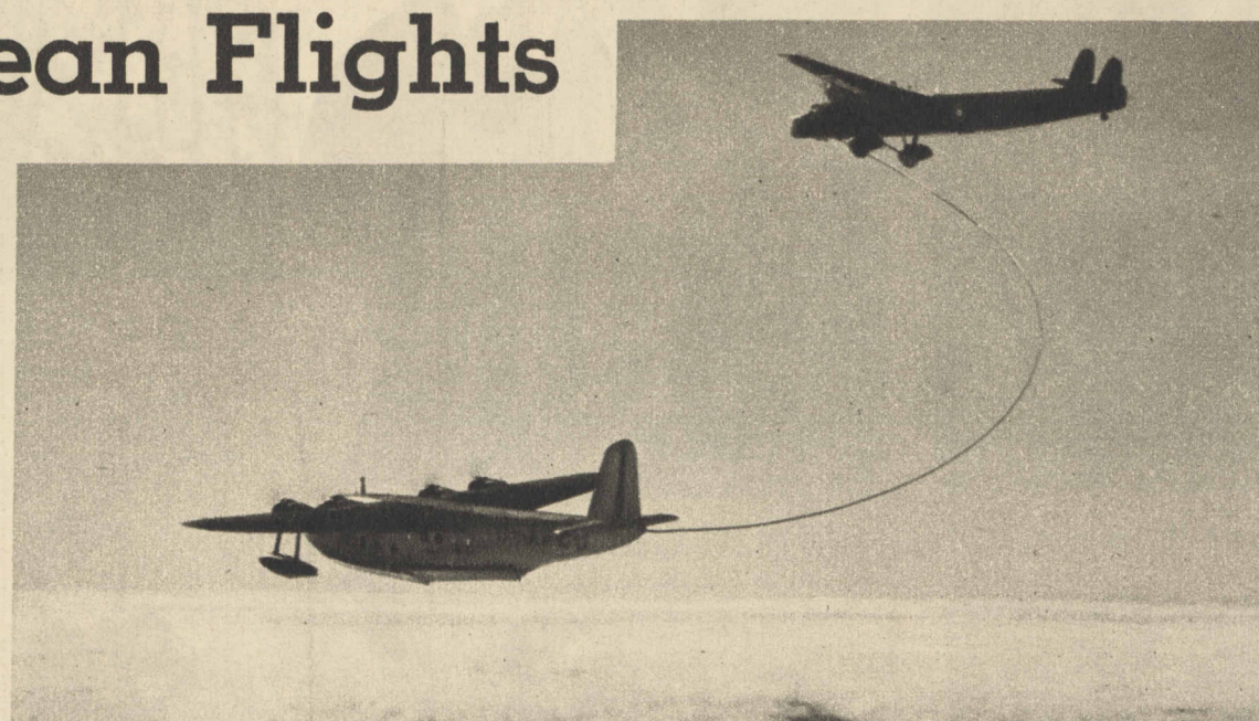
The Imperial flying boat Cabot receiving 1,000 gallons of fuel in midair from tanker.
